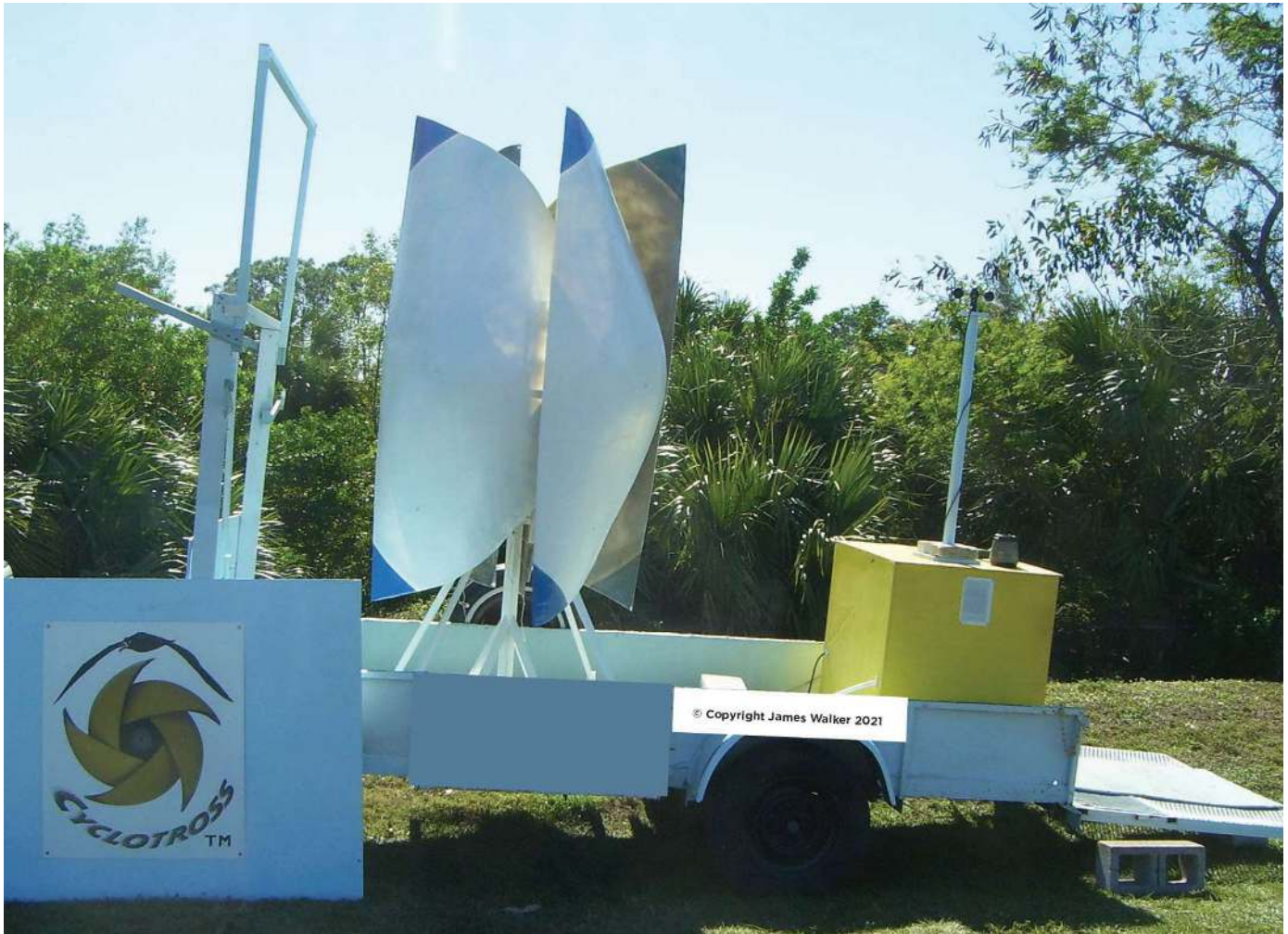
GRTC's previous smaller prototype success prompted the development of a larger device that could be trailer-mounted and transported to remote areas as a temporary or prolonged power station. (Courtesy: GRTC)
